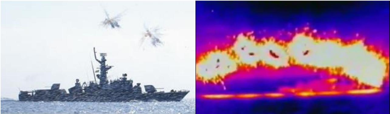
Figure 1 - Chaff<sup>2</sup> burst (left) and IR decoy<sup>3</sup> soft-kill countermeasures
