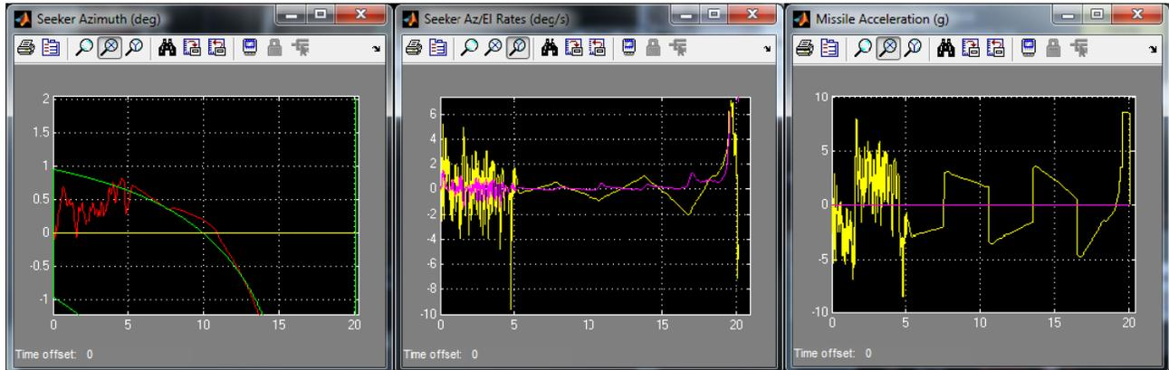
Figure 7 - Distraction decoy engagement results. Seeker Az angle (left), Az/El Rates (centre), Missile Body Accelerations (right)
