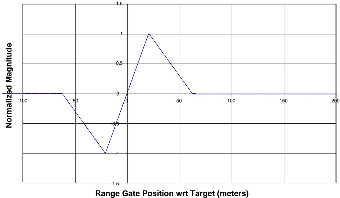
**Figure 1 Idealized Single Target Range Discriminator Curve**
